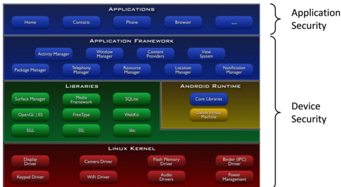
Fig. 2.3.1: Main Components of the Android Platform
