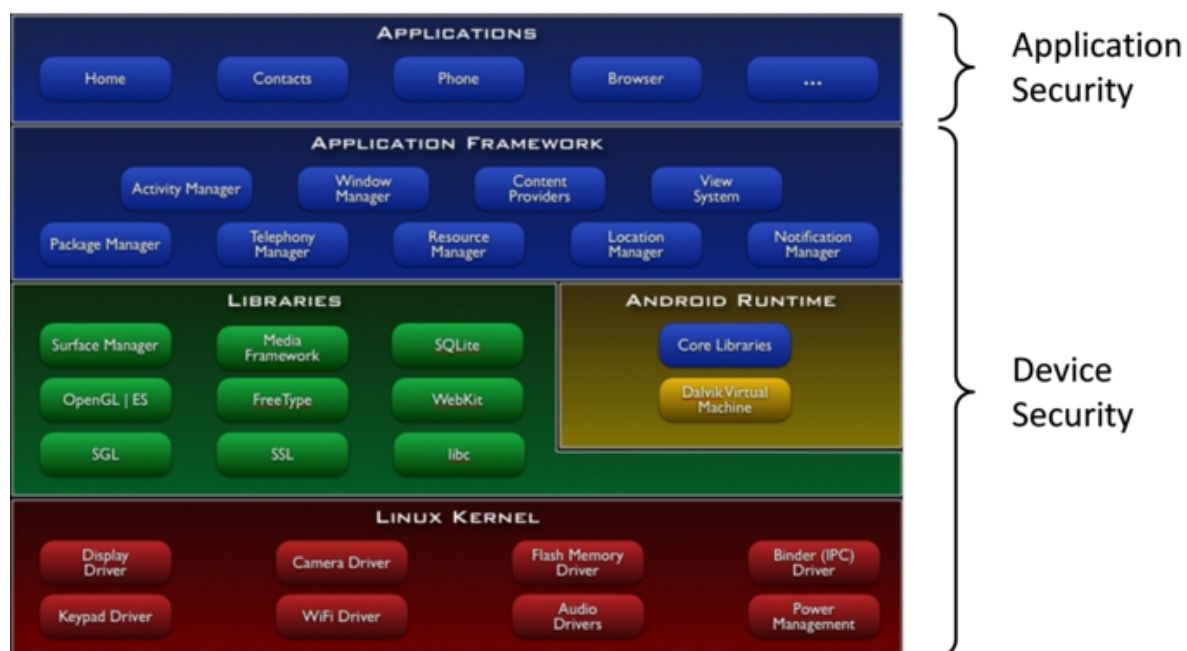
Fig. 2.3.1: Main Components of the Android Platform
