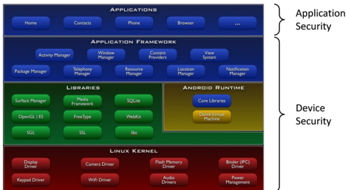
Fig. 2.3.1: Main Components of the Android Platform
